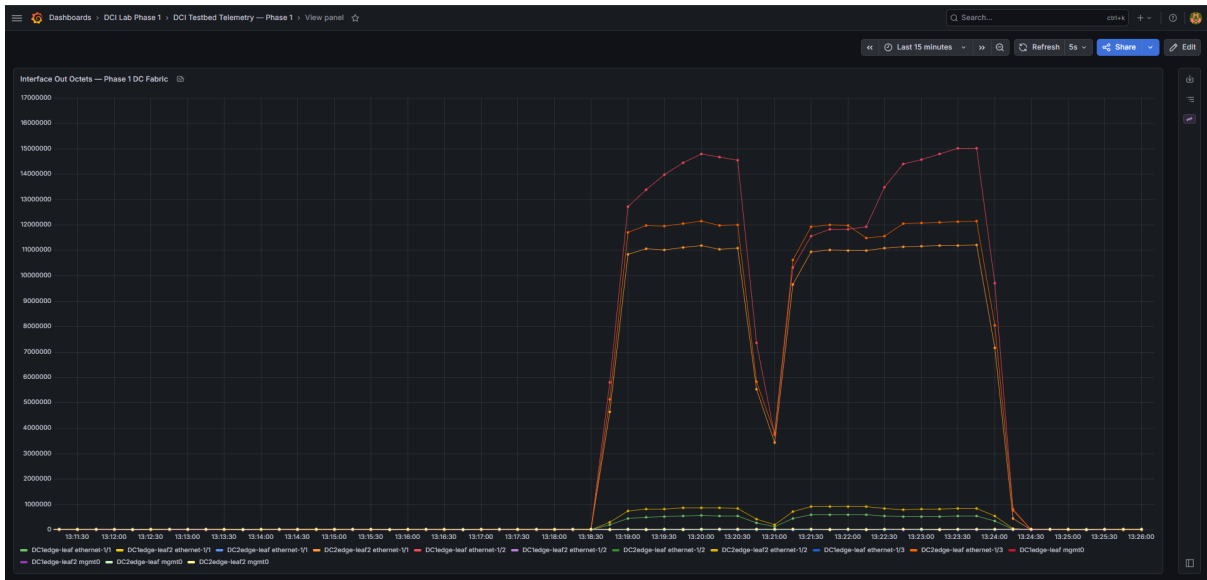
Figure 6.17: Phase 1 DC fabric interface activity (Grafana, “Interface Out Octets” panel, 15-minute window). Two traffic bursts are visible, each ramping to approximately 14–15.5 million octets; the dip between them corresponds to the IS-IS + LDP failure-injection event.
