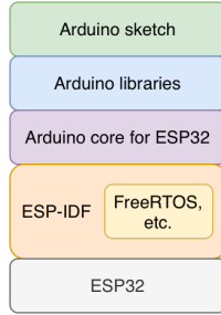
Fig. 1. Simplified software stack for running Arduino sketches on the ESP32, showing the Arduino core as a compatibility layer on top of ESP-IDF, which includes FreeRTOS, and the underlying hardware.
